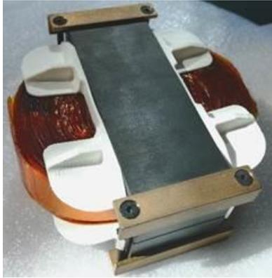
Fig. 3.2. Hardware prototype for the 20 kW, 100 kHz transformer
