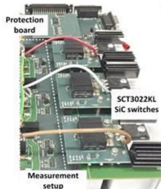
Fig. 3.1. Hardware prototype of a 20 kW PFC rectifier
