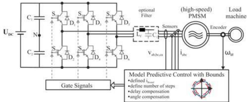
Figure 1: Schematic of 2-Level Voltage Source Converter with MPC
