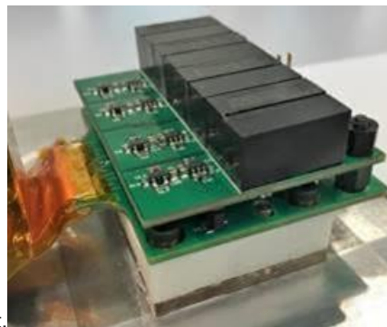
Fig. 3.2. Power module integrated with the drive circuit.
